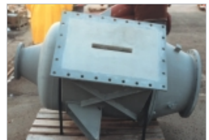
Hot gas cyclone at 1000 °C/1932 °F.
