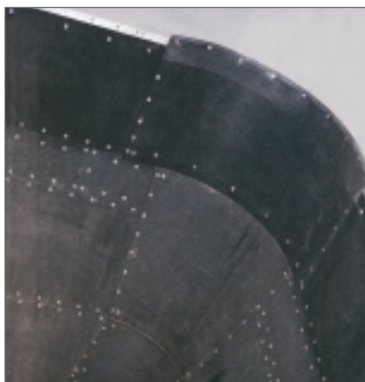
Shaped in a furnace, KALEN linings cut to size adapt themselves to curved surfaces.
