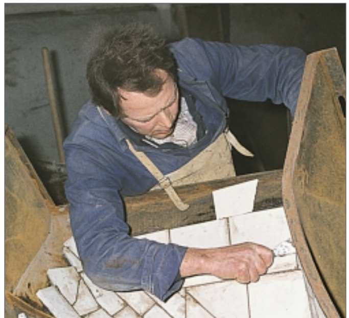
Chutes lined with KALCERAM are a solution that lasts, e.g. for bag loading systems in cement plants.
