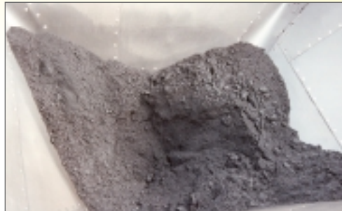
Bunker for fine coal: The slide-promoting lining ensures the material flow without sticking and clogging.
