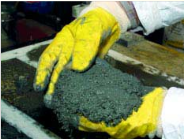
KALCRET compound must be sticky and allow plastic deformation.
