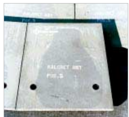
Lining of a vertical mill.
