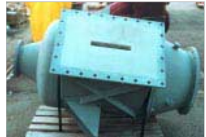
Hot gas cyclone at 1000 °C/1932 °F.
