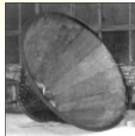
Cyclone with hardfaced lining for use at high temperatures.
