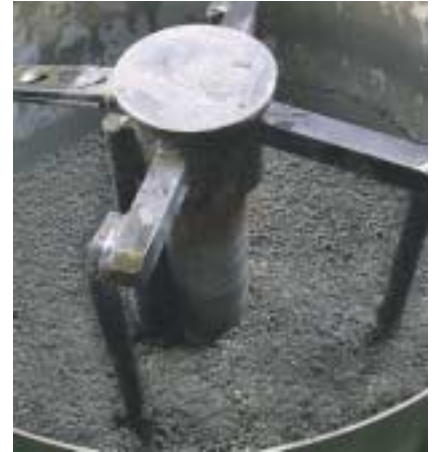
Mix for 5 minutes as specified; check result.
