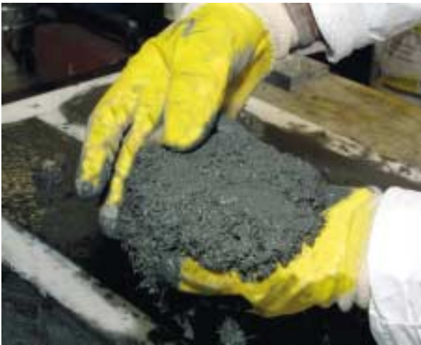
KALCRET compound must be sticky and allow plastic deformation.
