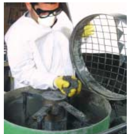
Continue mixing: for at least 2 minutes. Check result.
