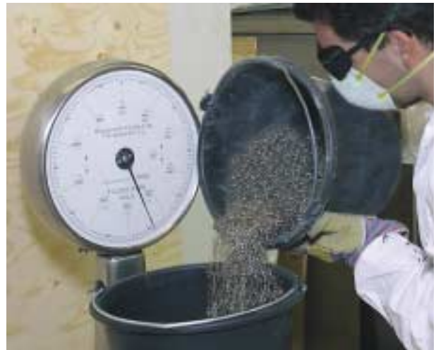
Kalenborn always recommends adding steel fibres.
